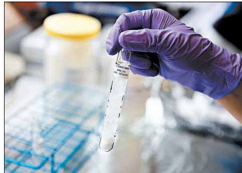
E. JASON WAMBSGANS/TRIBUNE PHOTO Mattress samples are prepared for testing to see if they contain flame retardants linked to increased cancer risk.
