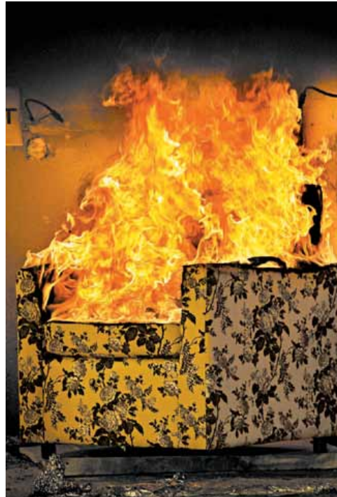
CONSUMER PRODUCT SAFETY COMMISSION PHOTO Up in flames: Government scientists found that chairs containing flame retardants, like the one being tested above, burned just as fast as identical chairs without them.
